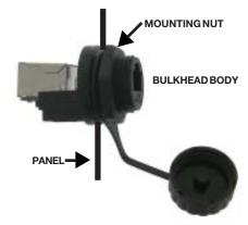
1: Mount Bulkhead Body with the Washer on the Outside, through Your Panel & Tighten Mounting Nut
